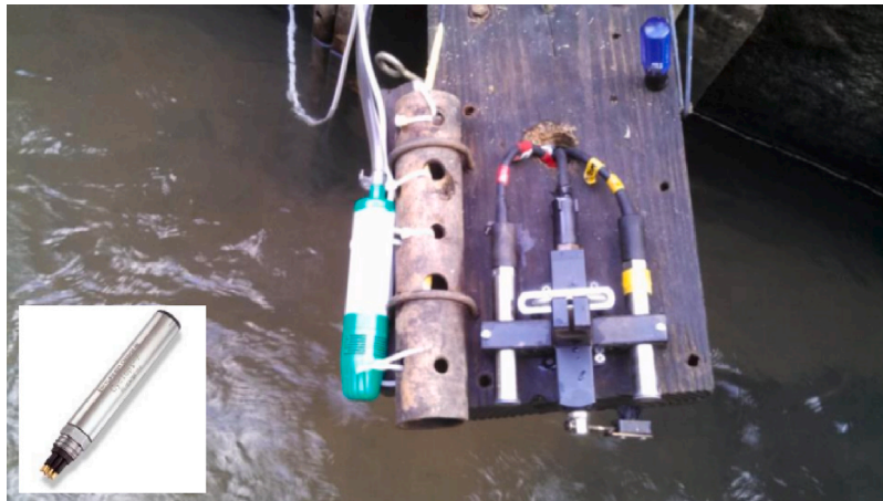
Fig. 1. Turbidity/fDOM sensor mounted on a board immersed in the water. The image in the corner is a Turner Designs Cyclops-7 submersible sensor (Lee et al., 2023).
